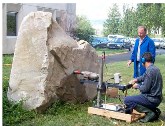
Figure 1: Drilling the block of granite C347, weighing 9500 kg
