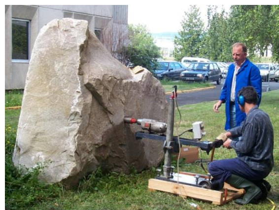
Figure 1: Drilling the block of granite C347, weighing 9500 kg
